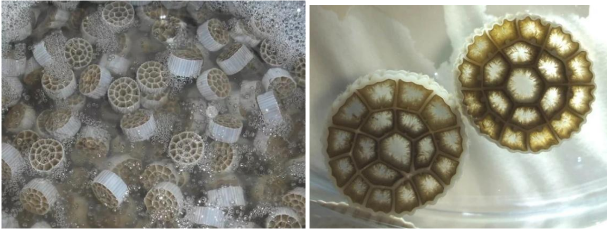
Figure 10-8: MBBR Media in Tank & Biofilm Growth on MBBR Media (Courtesy of Snowate)
